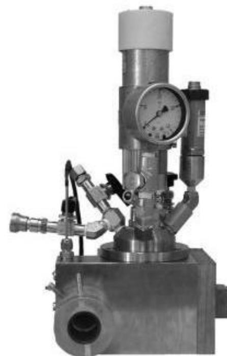
Figure 7.4 High pressure IR cell connected to an autoclave (constructed at ICCOM-CNR, 2003).
